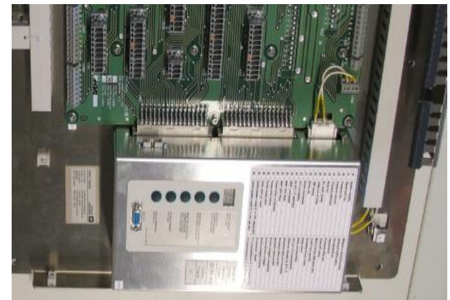
control panel in PCB technology, approx. 2h production time
